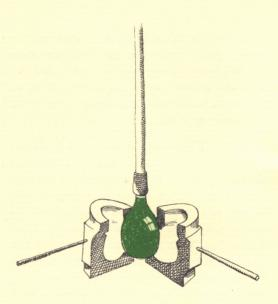
a rough shape on a marble slab. Then, blowpipe to lips, the glassmaker raised the pipe above his head, twirling the glass through the air in circles to create the shape he had in mind by centrifugal force. This free-blown method obviously required great skill—as well as time and lung power!
