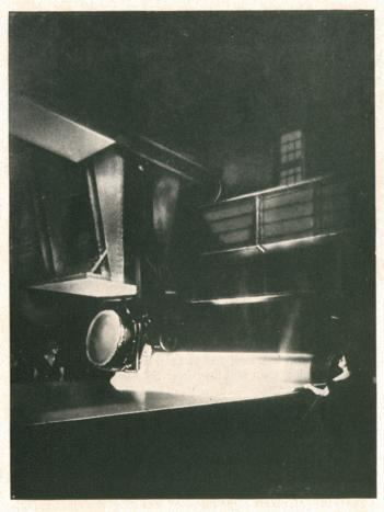
The pot, poised a moment above the casting table, is tilted so that the molten contents pour in a thick, dazzling flood across the table's width, and immediately the 25-ton steel roller moves forward, spreading out the molten mass before it as a cook rolls out dough
