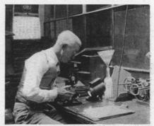
So many things can happen to a bottle in the process of manufacture that constant inspection is the only safeguard. This inspection is for strains and stresses which weaken the glass.
