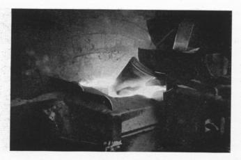
The sand, the soda ash and the other ingredients which go to make bottle glass are as carefully mixed as a housewife's cake. Only, of course, the measure is by the ton instead of by the ounce. Then it goes into the furnace, the mouth of which is shown here. It takes over 2500 degrees of heat to melt this mixture.
